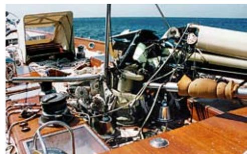
The 38m carbon in-mast furling rig collapsed when the 126ft ketch 'Hetairos' was hundreds of miles off New Zealand.
