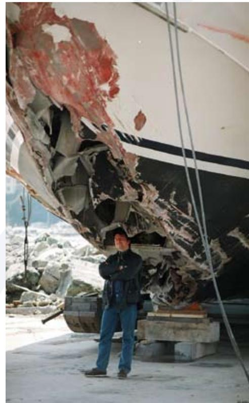
The 30m yacht hit rocks at full speed. A comprehensive, complicated survey of the whole hull structure was necessary as a result of the enormous impact.
